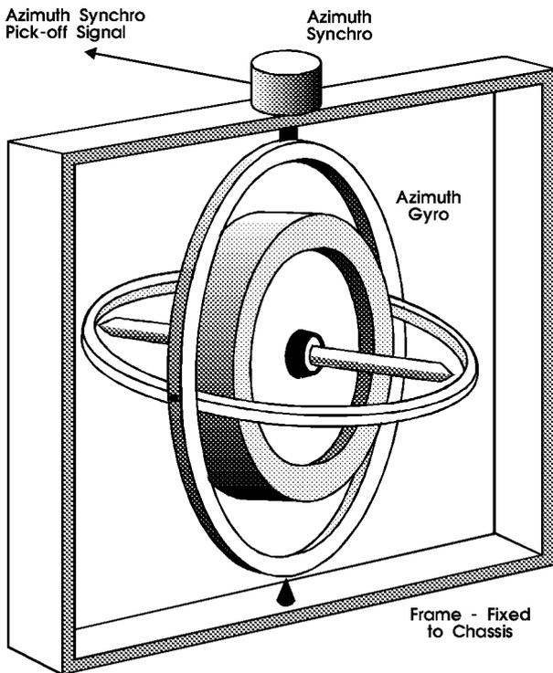
**Fig.4. The Azimuth Gyroscope**
