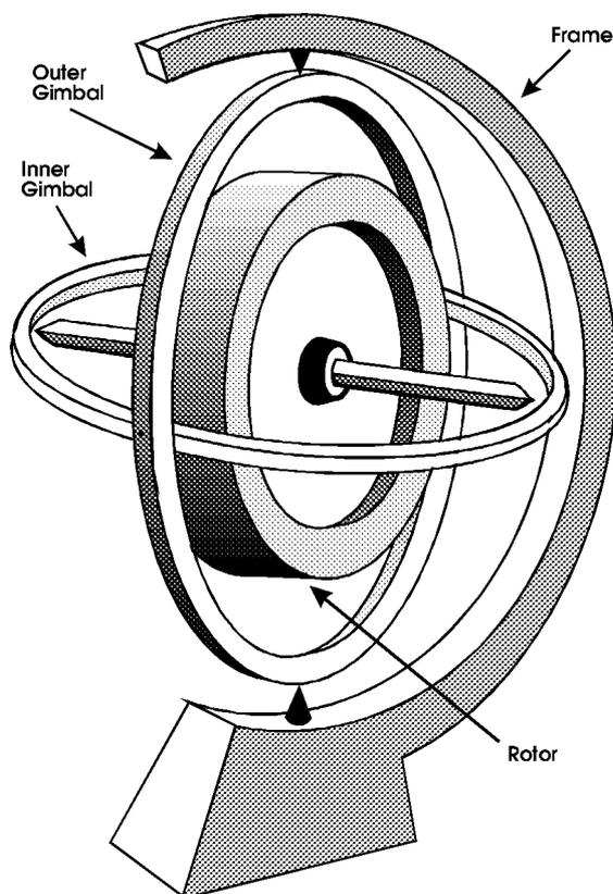
**Fig.1. The Displacement Gyroscope**
