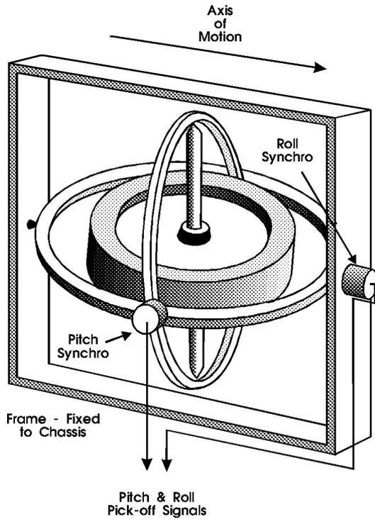
Fig.5. The Vertical Gyroscope
