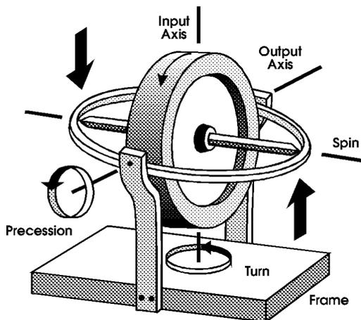
Fig.6 The Single Axis Gyroscope
