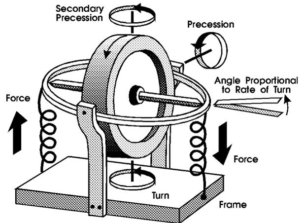
Fig.7. The Elementary Rate Gyroscope
