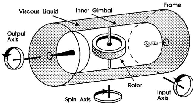
**Fig.9. The Rate Integrating Gyroscope**
